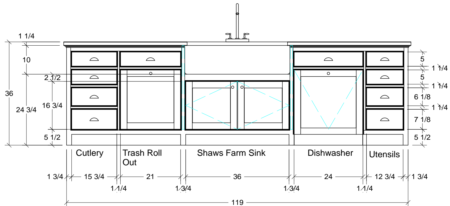
1 Elevation Kitchen Island - East Scale: 5/8" = 1'
